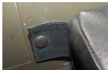
Rear cushion in Jason's Moke is held in with four press-studs to the body.
