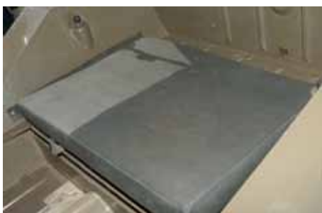
Rear cushion in Jason's Moke is held in with four press-studs to the body.
