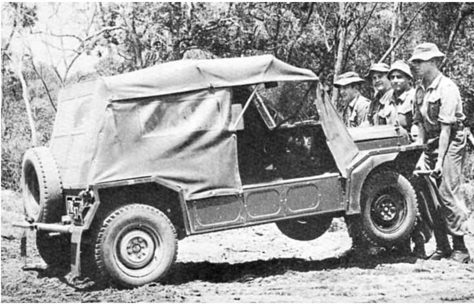
Ease of recovery is demonstrated with four soldiers lifting the front of the Moke...
