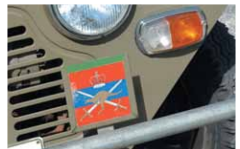
Front TAC-plate holder mounted to bumper.
